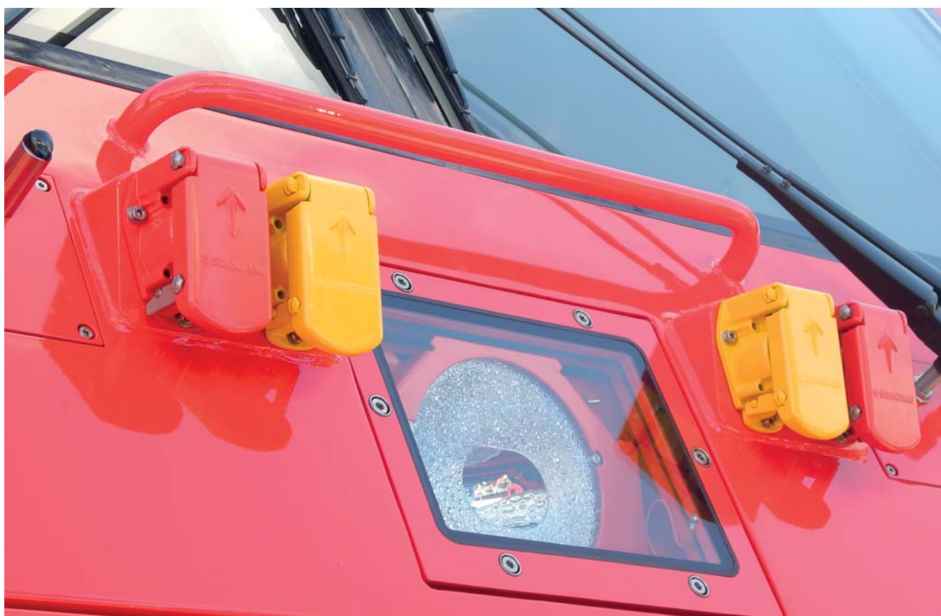
New UIC-IT connectors made by Schaltbau GmbH in TRAXX-model locomotives
